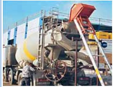
When integrating fiber into the truck mixer the fiber will not be uniformly distributed in the concrete. Therefore it's strongly recommended to integrate fiber in the mixer of the concrete plant!
