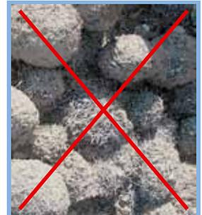
Dry balls in concrete due to wrong integration method and/or wrong concrete design.
