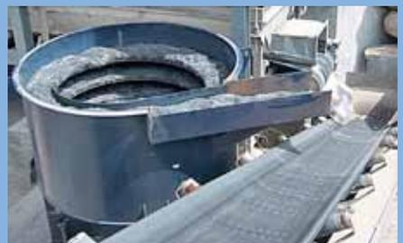
Cyclon system to dose fiber on conveyor belt
