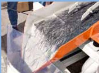
Vibration table of the blast machine to scatter the fiber before they fall into the airstream of the fiber blower
