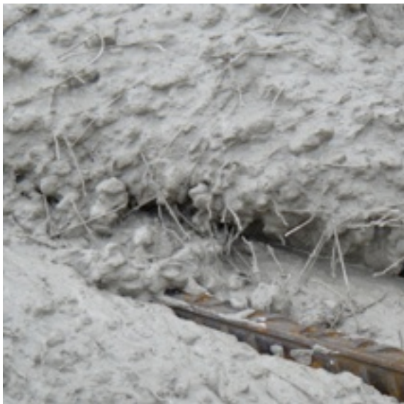
installation of APC-reinforcement in bottom layer on the day of casting concrete
